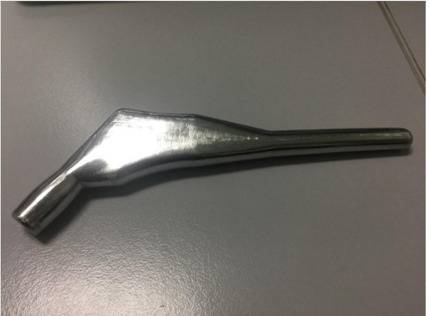
Figure 2: Successful printed hip femoral implant
