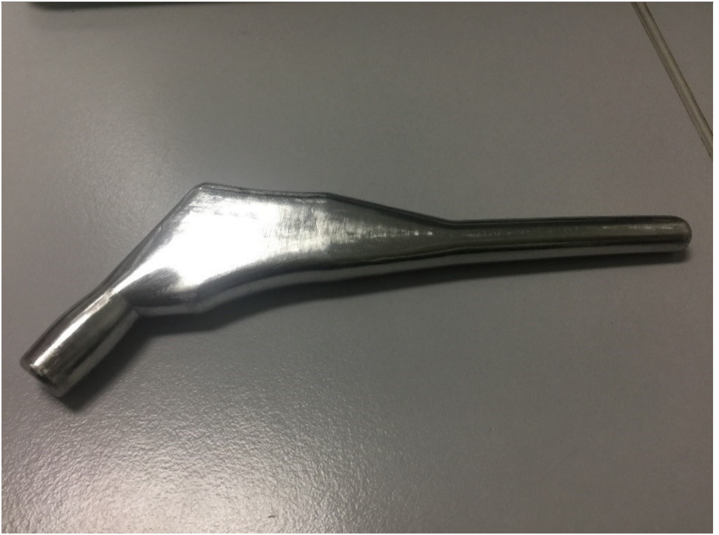
Figure 2: Successful printed hip femoral implant
