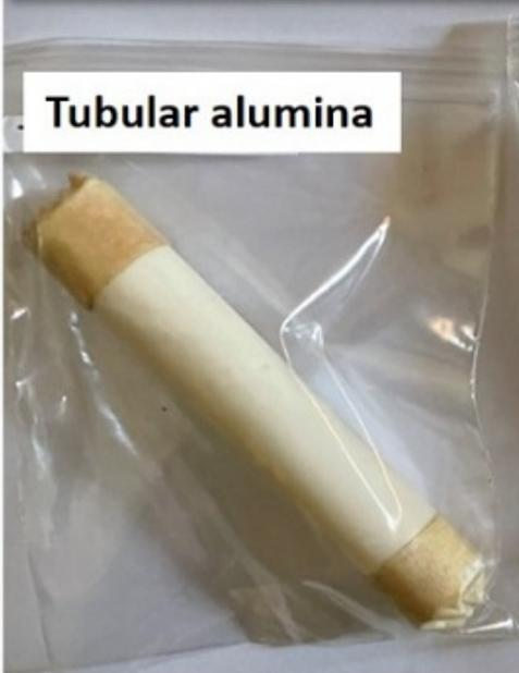
**Tubular-supported polymeric membrane**
