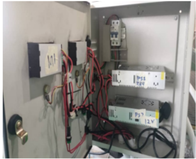
Figure 4: a) Electrical power box and (b) AC DC converter
