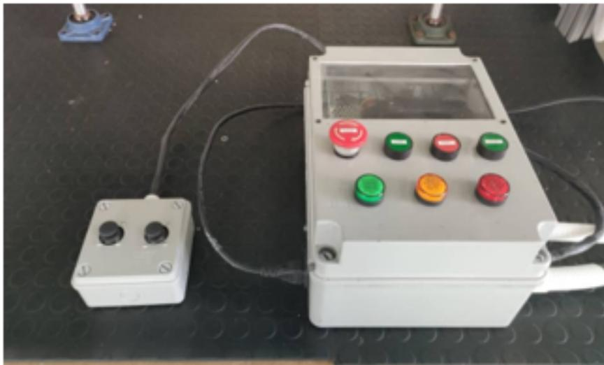
Figure 6: Joystick and PLC control box
