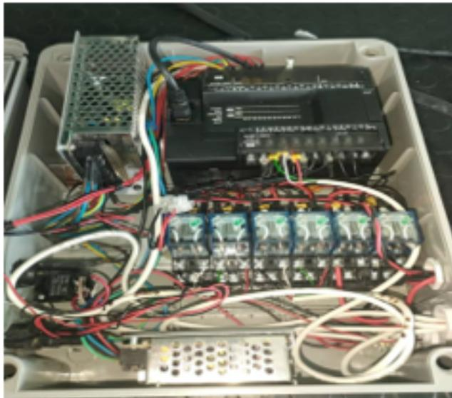
Figure 5: PLC and electronic components
