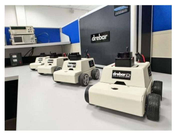
"It will communicate with DREBARbox and DREBAR OS to carry out advanced algorithmic functions such as Simultaneous Localisation and Mapping (SLAM), Obstacle Avoidance Module and others.
