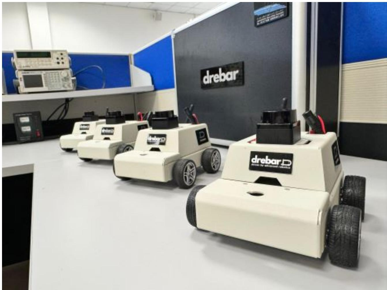
“It will communicate with DREBARbox and DREBAR OS to carry out advanced algorithmic functions such as Simultaneous Localisation and Mapping (SLAM), Obstacle Avoidance Module and others.
